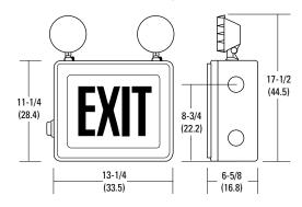
Mounting Tabs: Mounting enclosure to wall using (4) thru holes or optional mounting feet.
